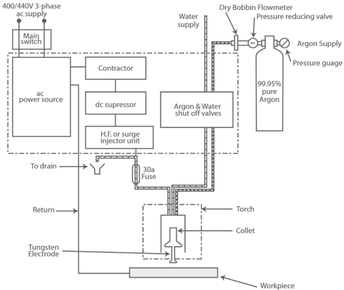
**Note:** Composite T.I.G. welding units include all the necessary auxiliaries. The argon and water shut off valves are usually controlled by solenoids, but may also be manually operated. The main power cable, fuse and torch can be air or water cooled.
