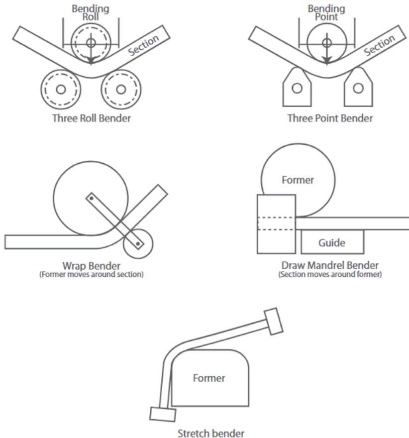
The three roll bender has a central moveable roller which is gradually depressed until the desired radius is obtained.
